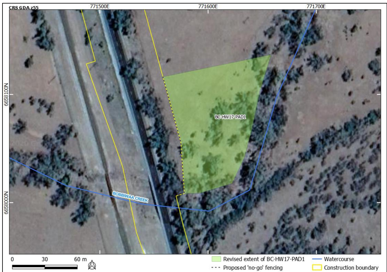
Figure 6-1: Revised extent of BC-HW17-PAD1 and the proposed 'no-go' zone fencing.
