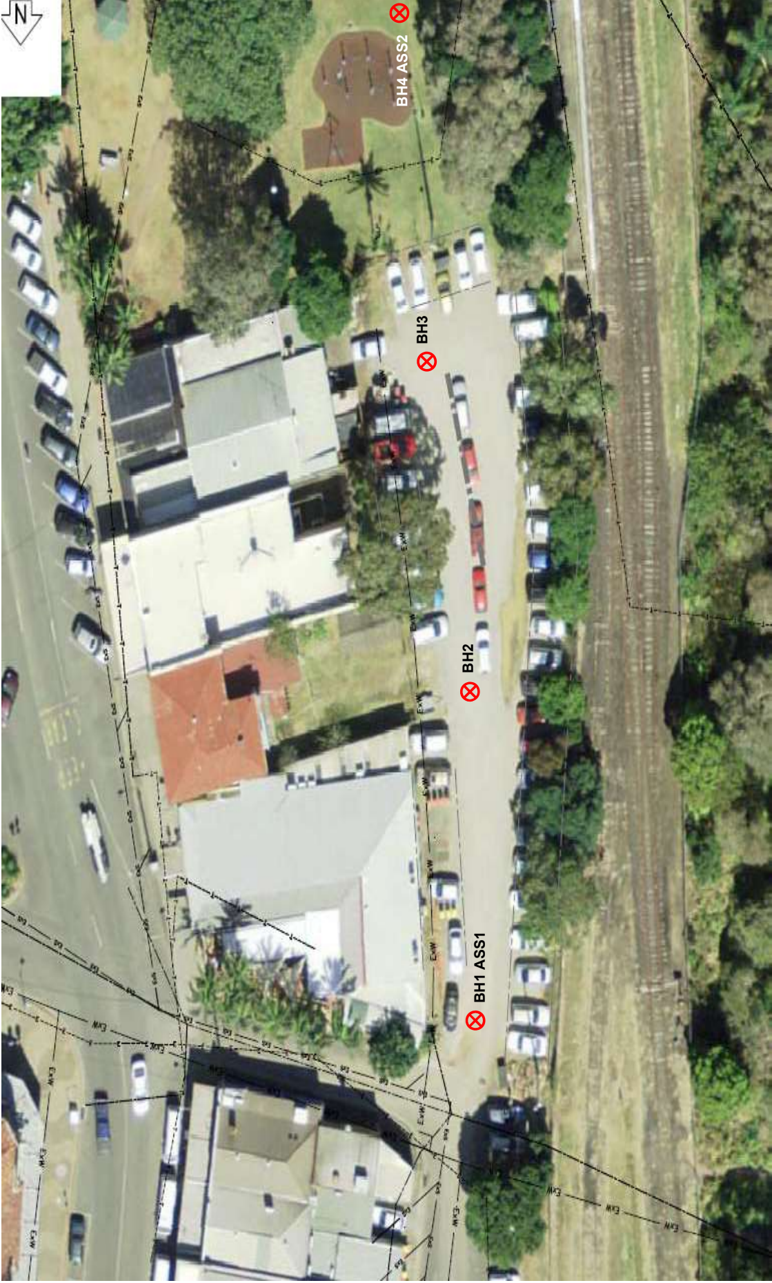
FIGURE 1: Sampling Plan – Soil Validation Lot 3 DP 827049 – Railway Hotel Carpark Imagery Courtesy of Six Maps 201
