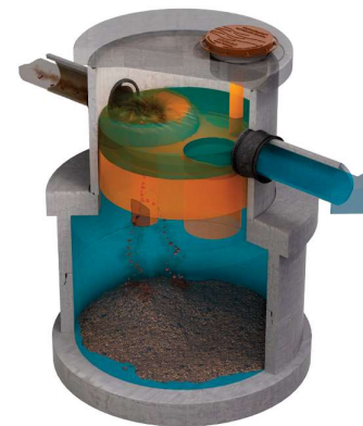
Figure 2 – HumeCeptor® system operation during high flow conditions
