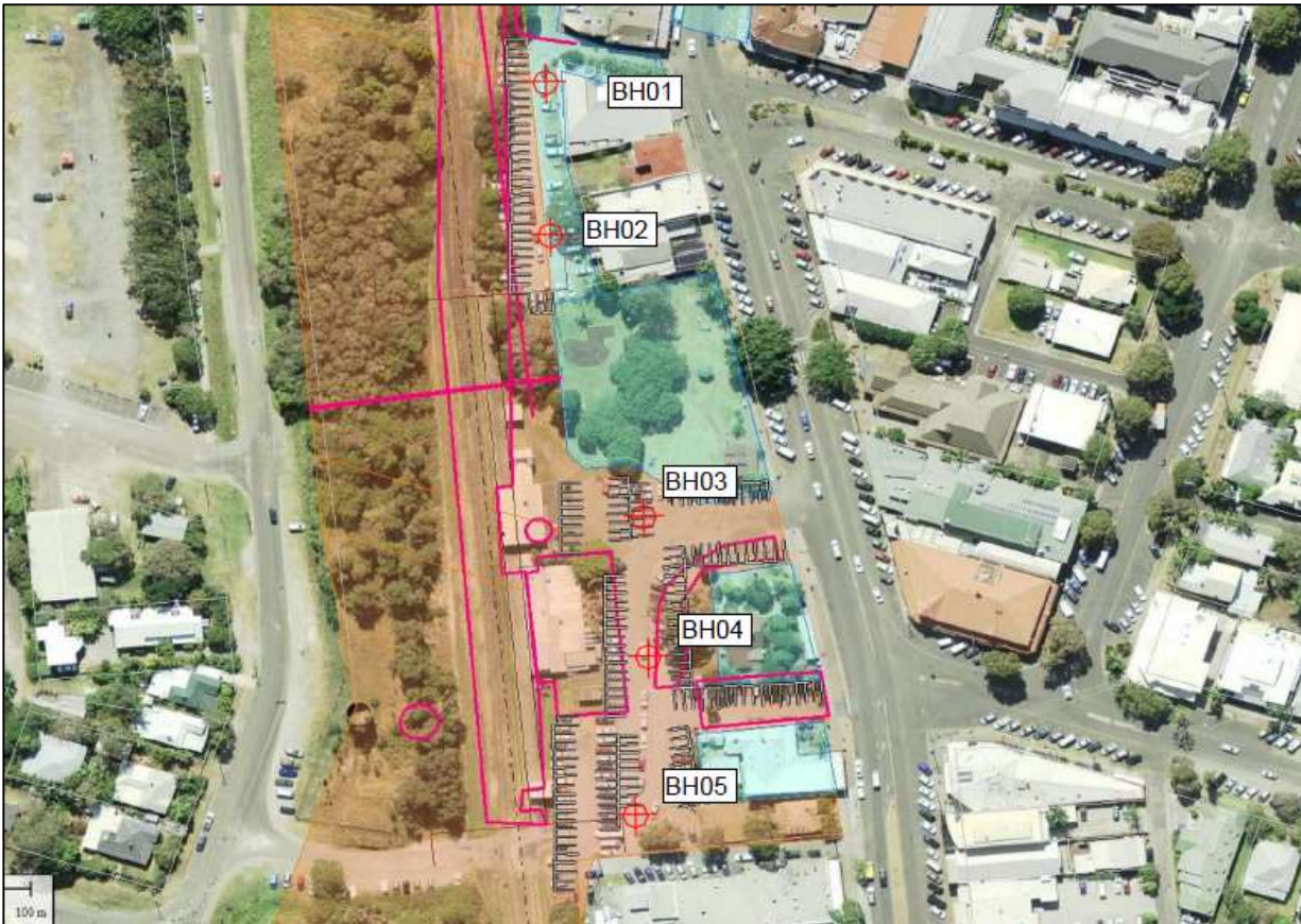
Figure 6: Aerial photograph showing borehole locations during geotechnical investigations.
