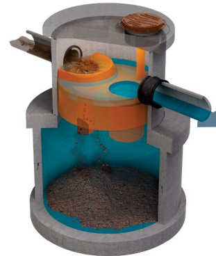
Figure 2 – HumeCeptor® system operation during high flow conditions
