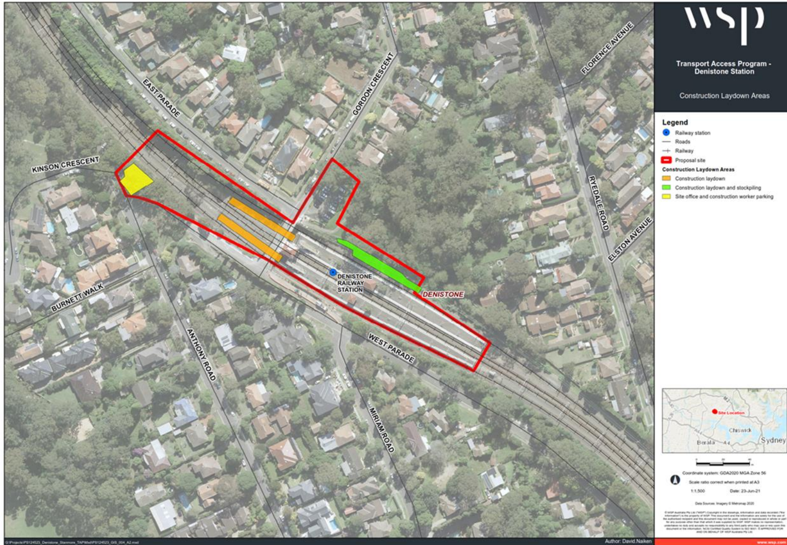
Figure 1.1 Construction compounds and laydown areas
