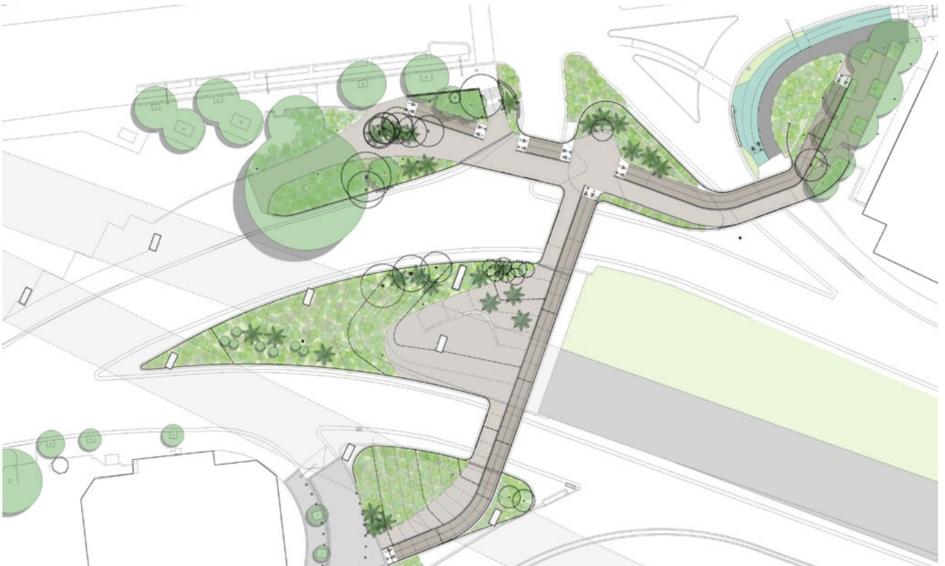
Kent Street underpass has clear direct connections either side of the under croft space. It also uses landscape to good effect improving the environment and providing shade and a cooler setting in summer.
