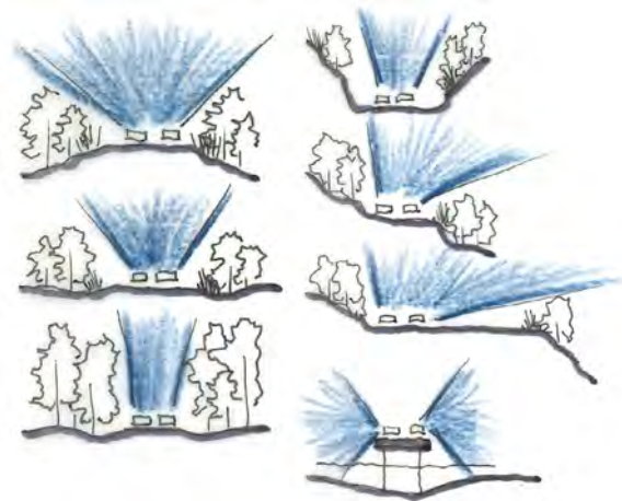
Figure 22—Modulating the ‘aperture’ of the roadway to the sky
